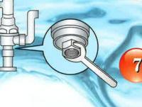
フランジ型安全弁の取付は、配管の無理な応力を避け るため必ずボルトは対角、交互に締めてください。 When installing a flange type safety valve, be sure to tighten bolts little by little and one after another in a diagonal position so as to prevent any stress a pipe.
